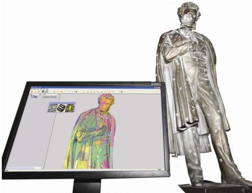
When you use markers or a rotary table, scanned elements are automatically aligned, which greatly simplifies the scanning process.
